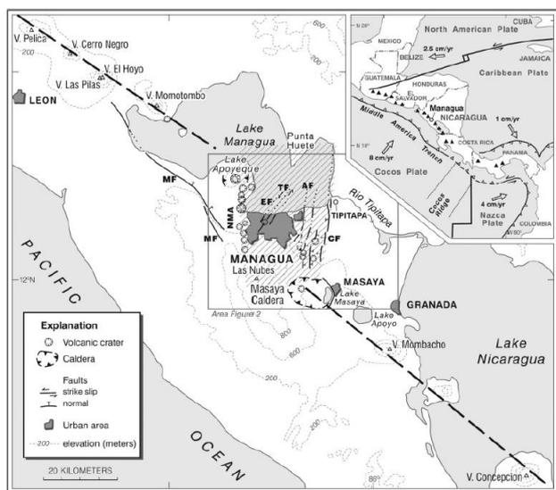
Figure 1. Map showing the major faults (MF, EF, TF, AF, GF) in and around the city of Managua, Nicaragua. The upper right corner shows the map of Central America, the tectonic plates and the volcanic chain (Cowan *et al.*, 2002).
