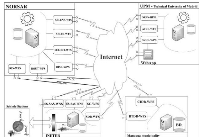
Figure 2. System architecture proposed for the web services
