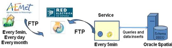
Figure 7. Data loading architecture
