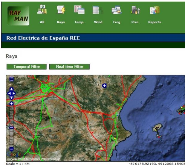
Figure 14. View of Web application interface based on GoogleMaps showing Ray information and the Electricity Network
