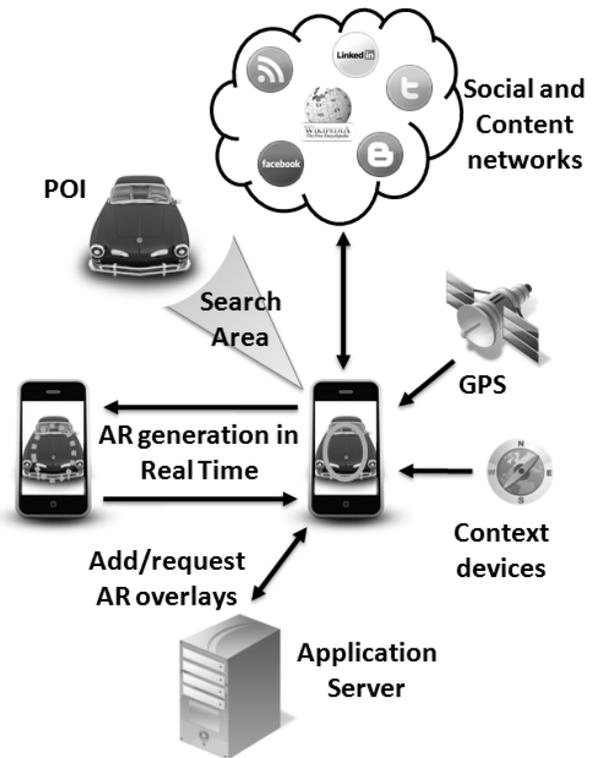
Figure 4. Live Level architecture.
