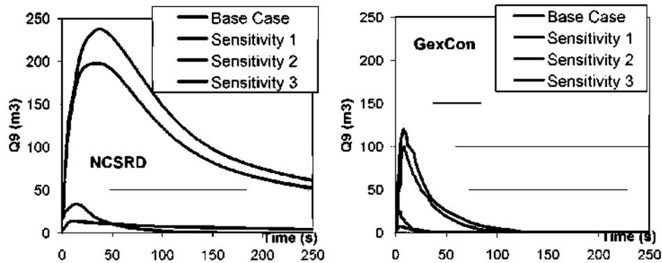
Fig. 10 – Equivalent stoichiometric cloud volume ( $Q_9$ ) predictions.
