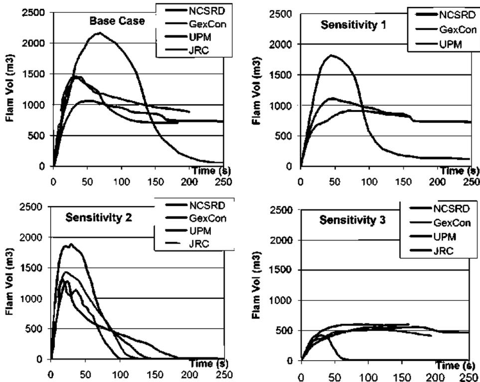
**Fig. 3 – Predicted flammable mixture volume ( $\text{m}^3$ ) histories per scenario case. Base case scenario: 20 kg of hydrogen was released in the basic geometry. Sensitivity Test 1: the hydrogen jet was moved to hit the light armature. Sensitivity Test 2: the underside of the bridge deck was flat. Sensitivity Test 3: the release was from one cylinder instead of four (5 kg instead of 20 kg).**
