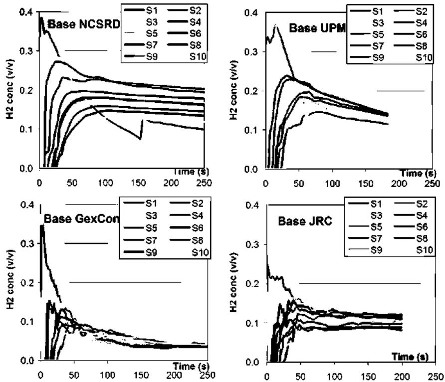
Fig. 4 – Base case: predicted hydrogen concentration time histories at sensors (1–10) locations.
