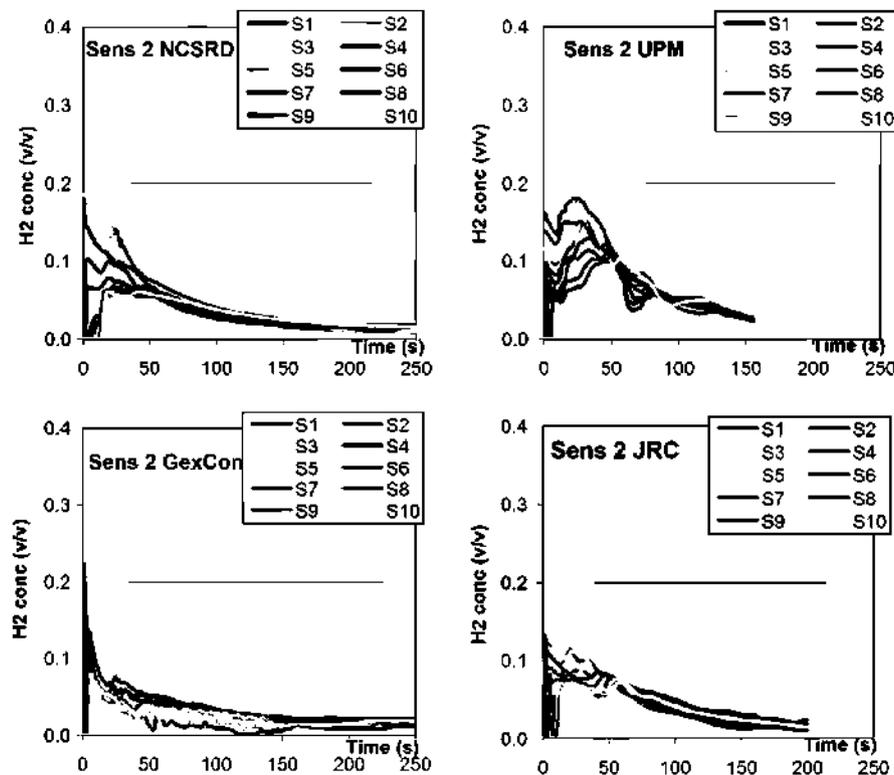
**Fig. 7 – Sensitivity test 2 (flat roof at  $z = 5$  m): predicted hydrogen concentration time histories at sensors (1–10) locations.**
