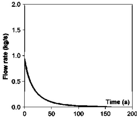
**Fig. 2 – Predicted mass flow rate for 20 kg hydrogen release at 35 MPa, ambient temperature from 4×4 mm diameter nozzles.**
