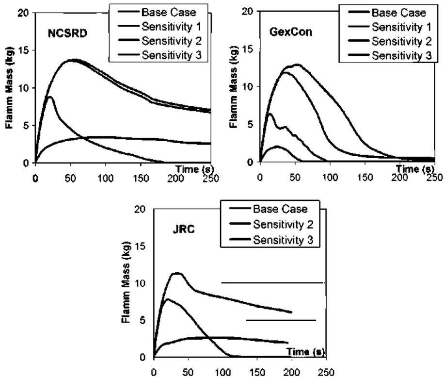
Fig. 9 - Flammable hydrogen mass predictions.
