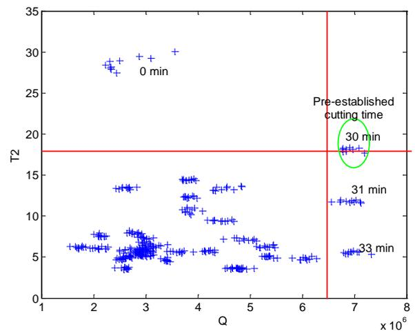
**Figure 6.** Biplot of Q vs T2 statistics of the PCA model developed for sheep milk coagulation process. Red lines indicate the T2 limit (horizontal) and Q limit (vertical).
