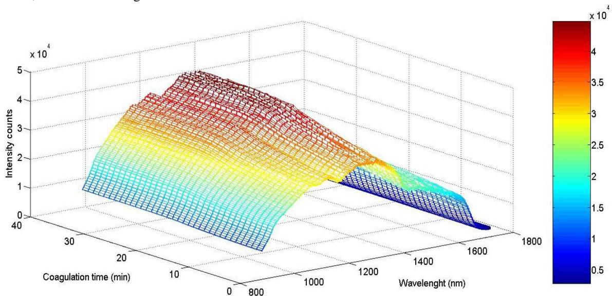
**Figure 3.** Surface graphic for light intensity recovered for each wavelength and coagulation time. Color bar represents the intensity counts values.
