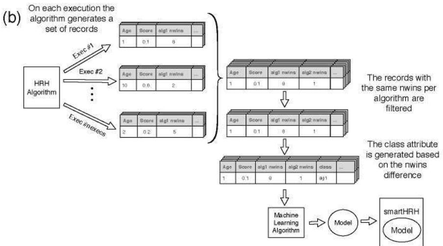
Fig. 1. Generation of the data records and learning procedure
