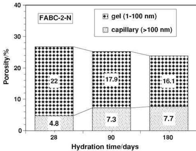
**Fig. 3** Evolution of gel and capillary porosity of FABC-2-N hydrated cement calculated from N<sub>2</sub> adsorption isotherm (1–100 nm) and mercury intrusion porosimetry (>100 nm)
