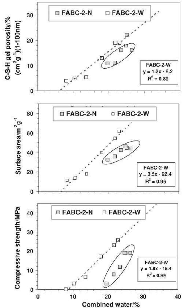
**Fig. 6** Quantitative correlations among combined water and: compressive strength, surface area and porosity of C-S-H gel. Influence of type of belite cement
