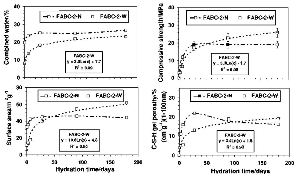
The decrease in C-S-H porosity is accompanied by an increase in the amount of the capillary pores (>100 nm), as can be seen in Fig. 3 (from 4.8% to 7.7%), justifying the loss of mechanical strength observed in Fig. 2. The presence of larger capillary pores was also suggested by SEM (Fig. 4), in which compact C-S-H gel blocks of FABC-2-N that were hydrated for 180 days appeared together with micro cracks (capillary pores).
