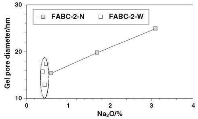
**Fig. 5** Correlation of the percentage of Na (expressed as Na<sub>2</sub>O) of the C-S-H gel and the average gel pore-diameter. Influence of type of belite cement
