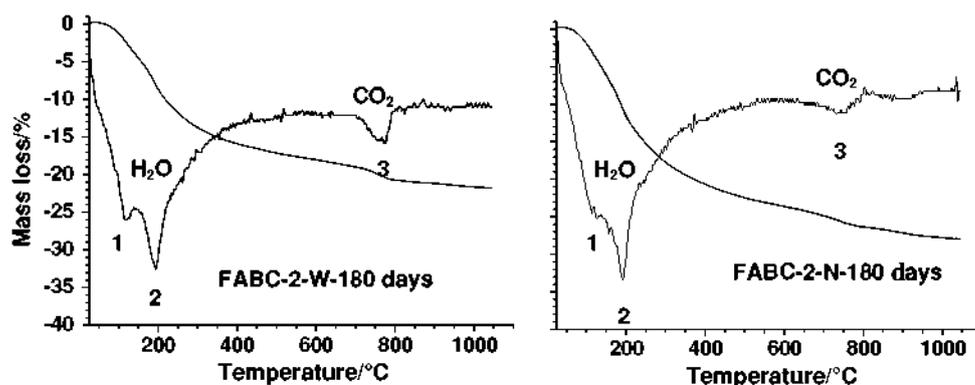
the TG curves, which is due to the release of water from the hydrated products. In the corresponding DTG curves, two maxima are observed at 100 and 200 °C. A second mass loss is also observed between 700 and 1,100 °C, due to the release of CO<sub>2</sub> during calcite decomposition, which produces a DTG peak centred at 750–800 °C. Some of the CaCO<sub>3</sub> content was already present in the anhydrous FABC. This second mass loss was not considered for calculating the combined water.
