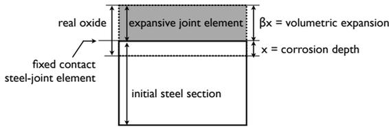
Figure 1: Sketch of the expansive joint element
