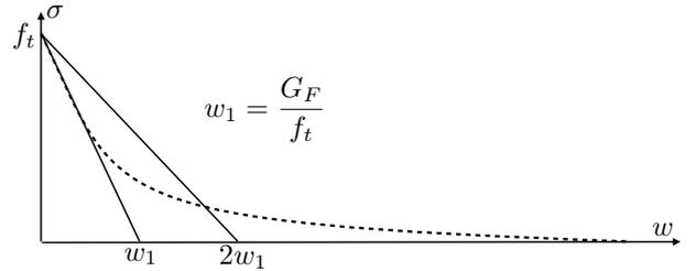
Figure 2: Sketch of the curvilinear softening curve, and the two linear approximation used in the paper
