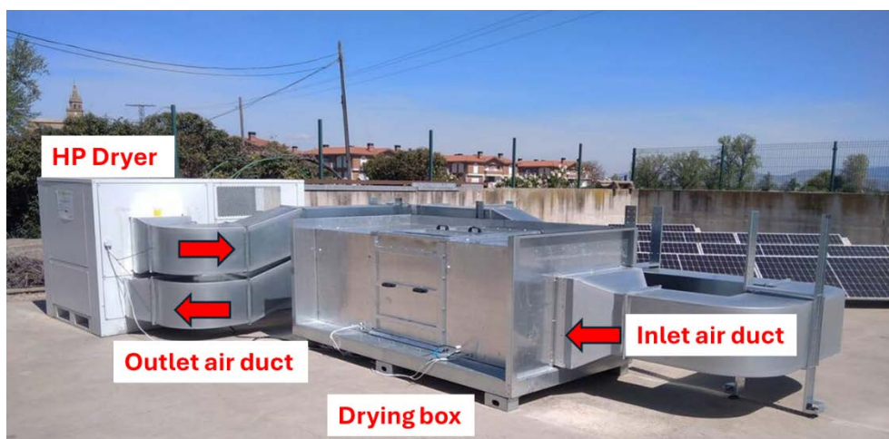
Figure 21: Drying infrastructure of the prototype of 2023. It consists of an HP dryer unit (which extracts humidity from the air), the inlet and outlet aluminum air ducts and the drying box (where the alfalfa bale is). The red arrows indicate the air flow direction.
