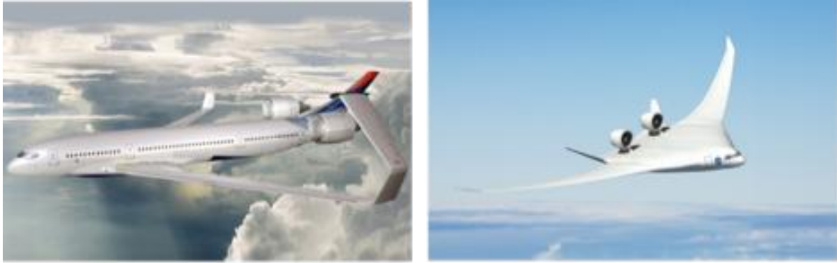
Figure 4-7: examples of revolutionary unconventional aeroplane configurations. (a) Left-hand-side image: box wing configuration example from Lockheed Martin (image from commons.wikimedia.org). (b) Right-hand-side image: BWB configuration from Boeing-NASA (image from commons.wikimedia.org).
