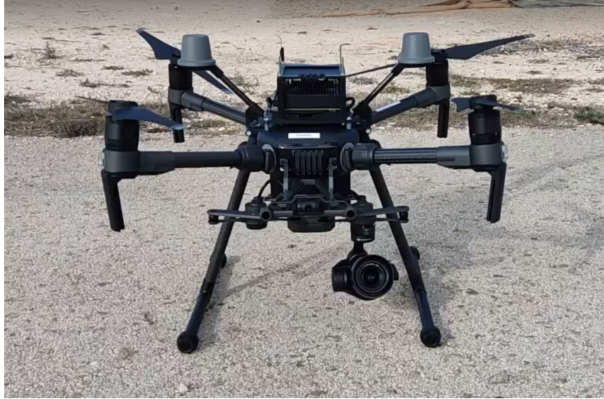
Figure B.4: DJI Matrice 210 V2 Equipped with the Nvidia Jetson AGX XavierSBC
