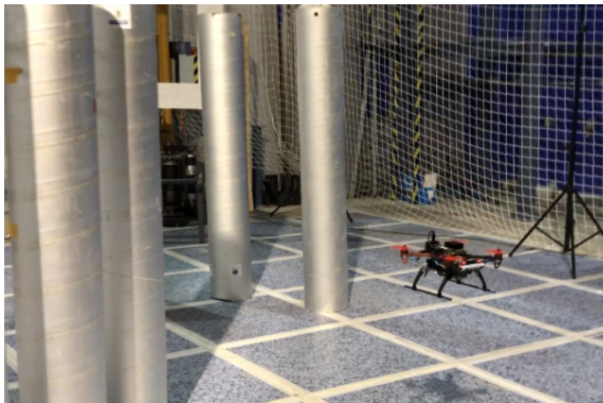
Figure 8.4: Experimental setup used to validate the proposed solution. The drone must navigate in a scenario with a set of columns.
