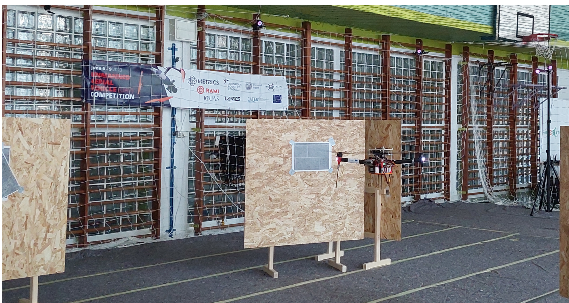
Figure 8.23: Real environment scenario with the drone flying while searching for defects.
