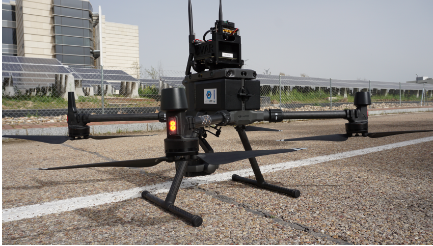
Figure B.5: DJI Matrice 300 RTK Equipped with the Nvidia Jetson AGX XavierSBC
