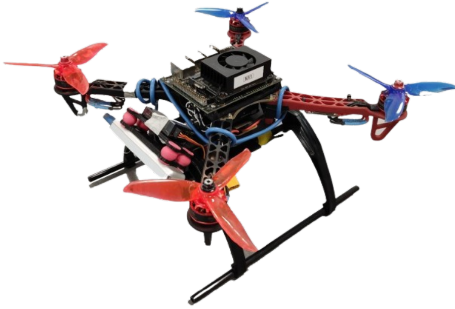
Figure B.3: Custom F330 based quadrotor equipped with an NVIDIA Jetson Xavier NX, a Pixhawk 4 Mini, an Intel RealSense T265, and a USB fisheye camera.
