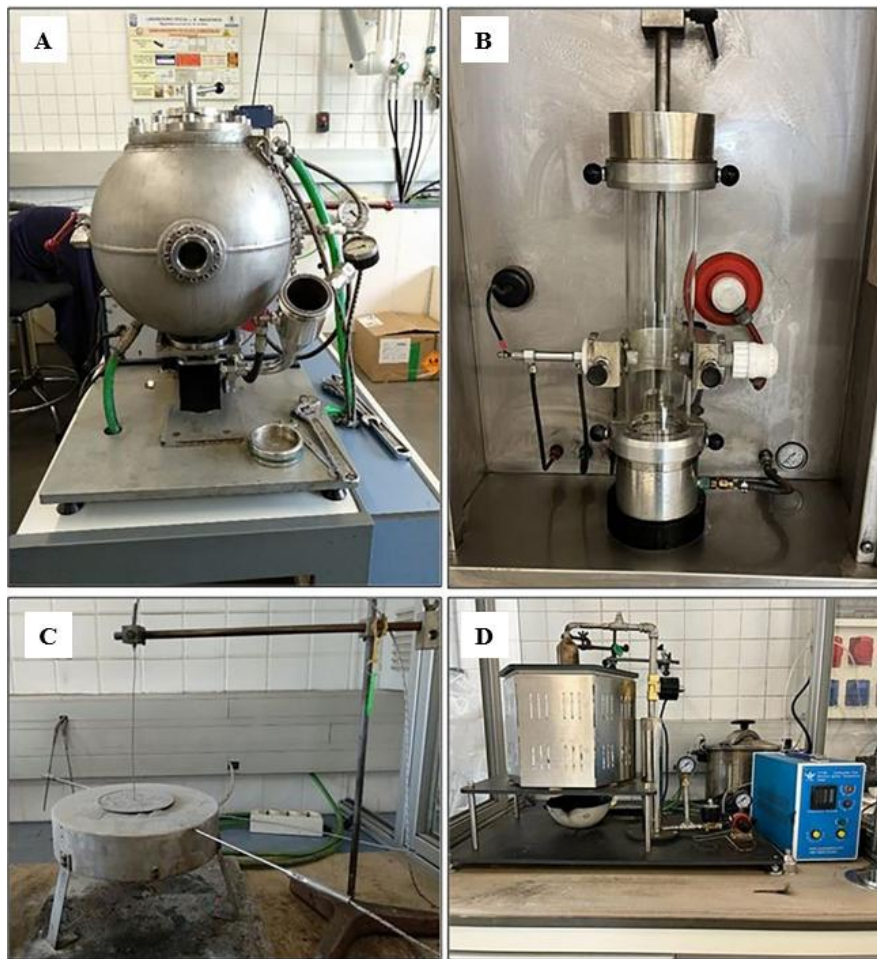
Figure 1.9: a) Severity test apparatus (20 litres sphere), b) minimum ignition energy test apparatus (Hartmann tube), c) minimum ignition temperature of dust layer test apparatus and d) minimum ignition temperature of dust cloud test apparatus (G-G furnace) [68]
