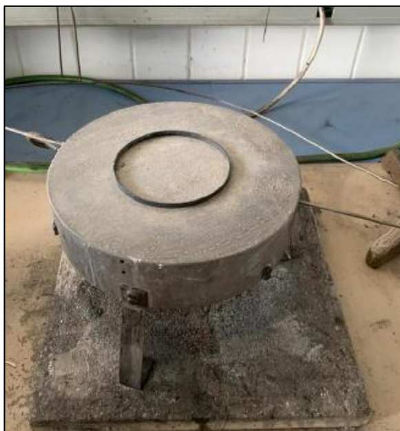
Figure 2.7. Minimum ignition temperature of dust layer apparatus
