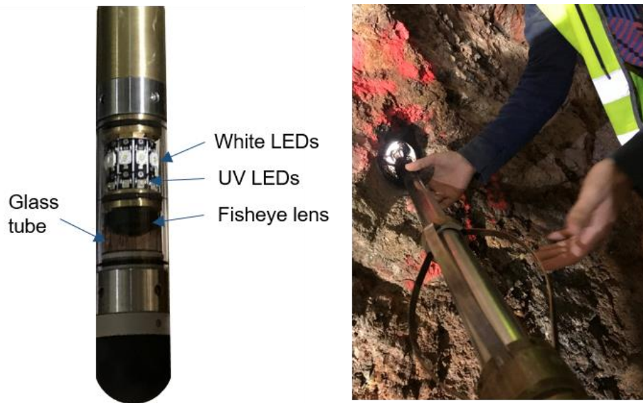
Figure 42. Bottom part of the logging tool (left) and final stages of borehole surveying with the forward centralizer and the glass tube inside the hole (right).
