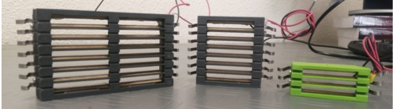
Figure 3.3: Various designs of atmospheric plasma devices based on the described geometry.
