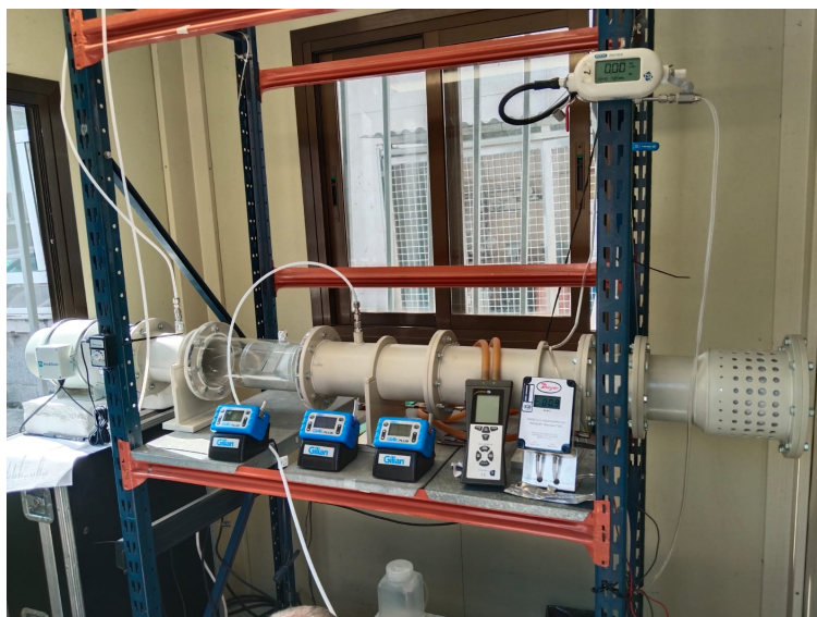
Figure 8.1: Experimental setup for the evaluation of the efficacy of ANTP against VOCs.
