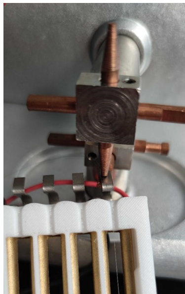
Figure 3.8: Microwelding process using a plasma device.
