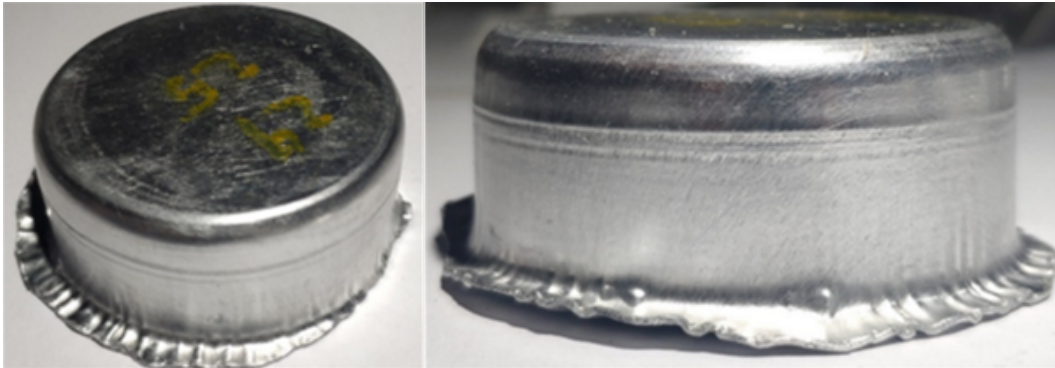
Figure 7.24: Sheet metal forming validation. Cylindrical shape formed using a Tough PLA matrix using 0.5[mm] thickness AW1050 aluminum sheet.
