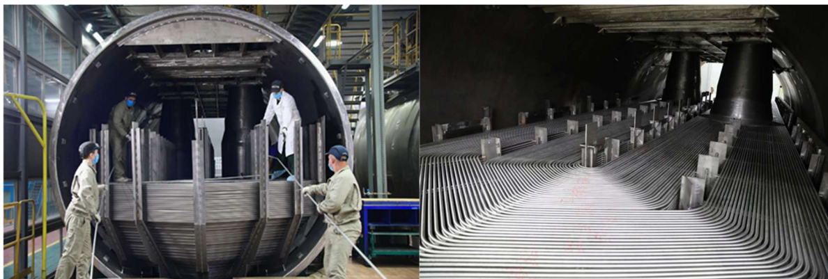
Figure 2-17 VVER-1000/V320 SGs U-shaped tubes
