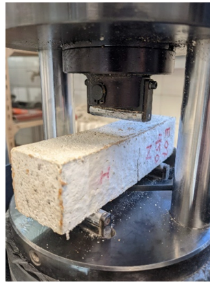
Fig. 10. Specimen E0.7-450-N after flexural strength test.
