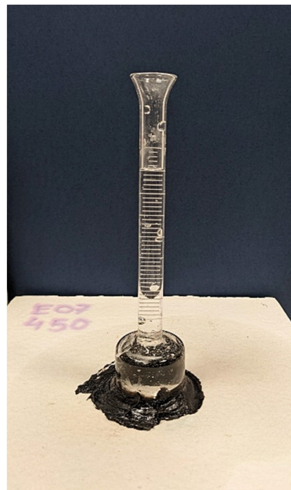
Fig. 5. Karsten Tube Penetration Test.
