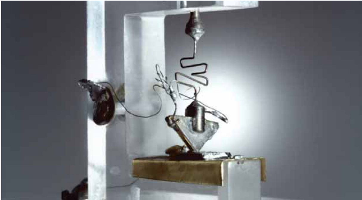
Figure 35. First Transistor device. 1947
