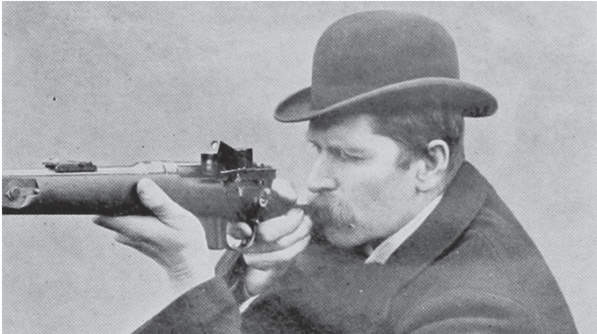
Figure 46. The Reflector Sight. Howard Grubb. 1900.
