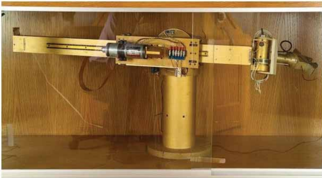
Figure 32. First 6 Axis Robot. Victor Scheinman. 1969.
