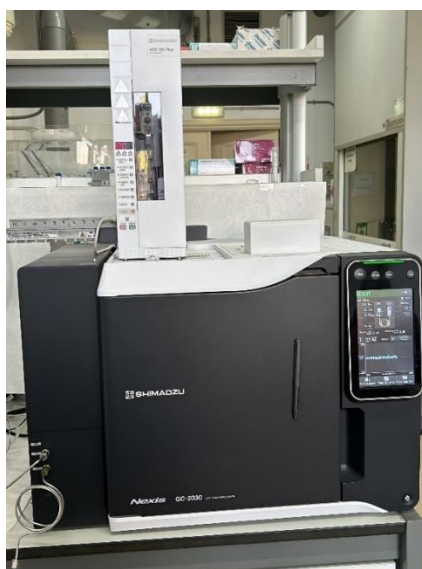
Figure 5.21 Image of the gas chromatograph available at the ICP-CSIC, used to analyze the production of formic acid in our three-chamber electrolyzer.
