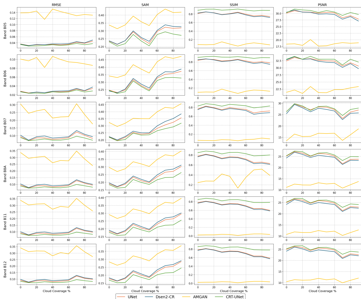
Figure 4.12: Quantitative performance of CRT-UNet and baseline models (UNet, DSen2-CR, AMGAN) across different cloud coverage levels for Sentinel-2 bands at 20 m resolution.
