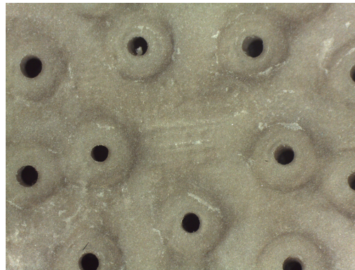
Figure 5.29: Case 7 panel made of PEEK, with different perforation diameters.
