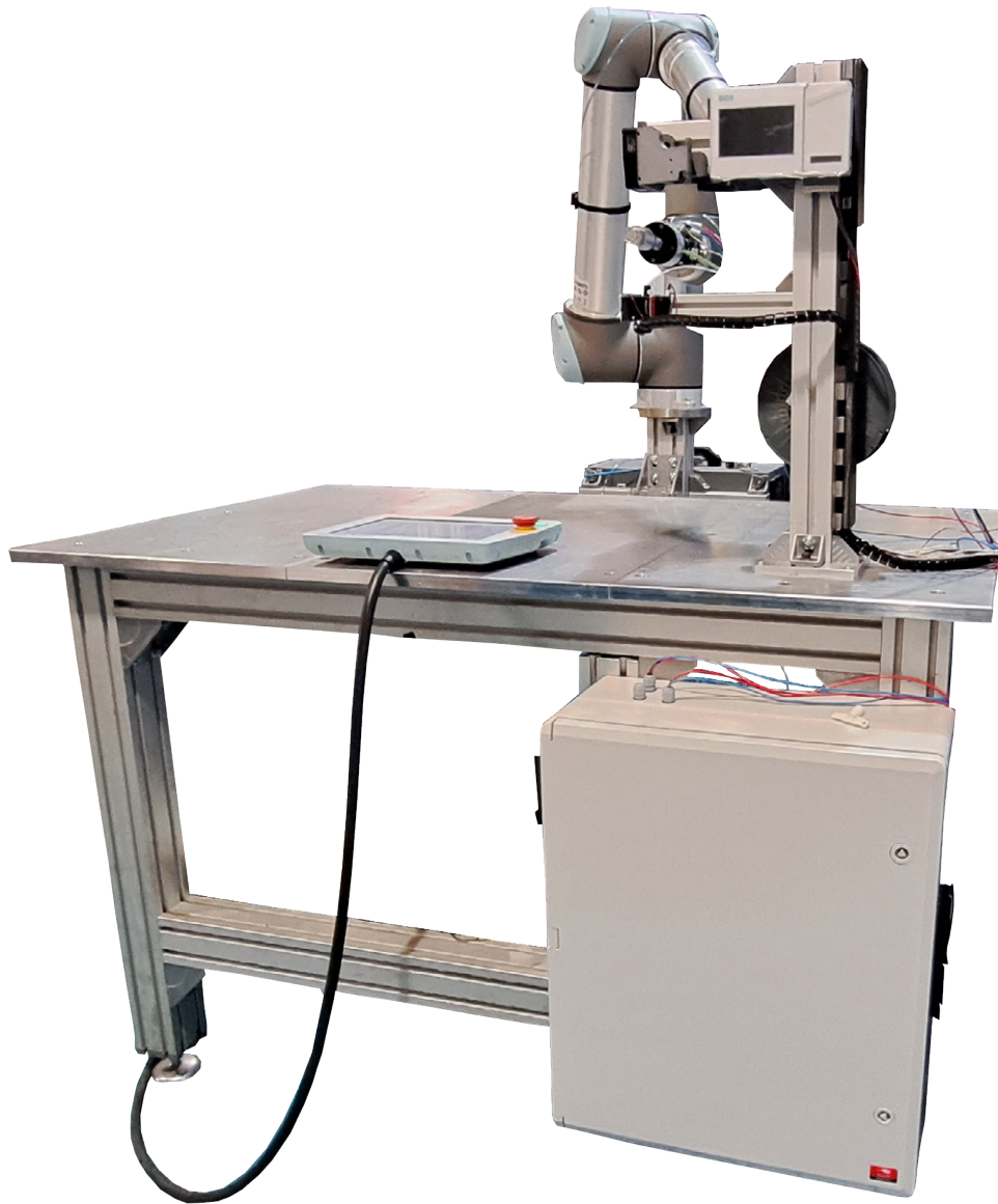
Figure 6.29: Robot-based NPAM-MEX-P manufacturing cell developed in this Thesis (front view).
