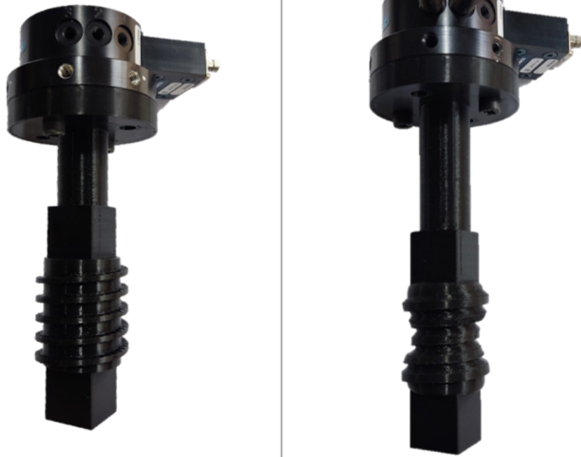
Figure 7.12: Cylindrical spring on top of its build platform (left), hourglass spring on top of its build platform (right).
