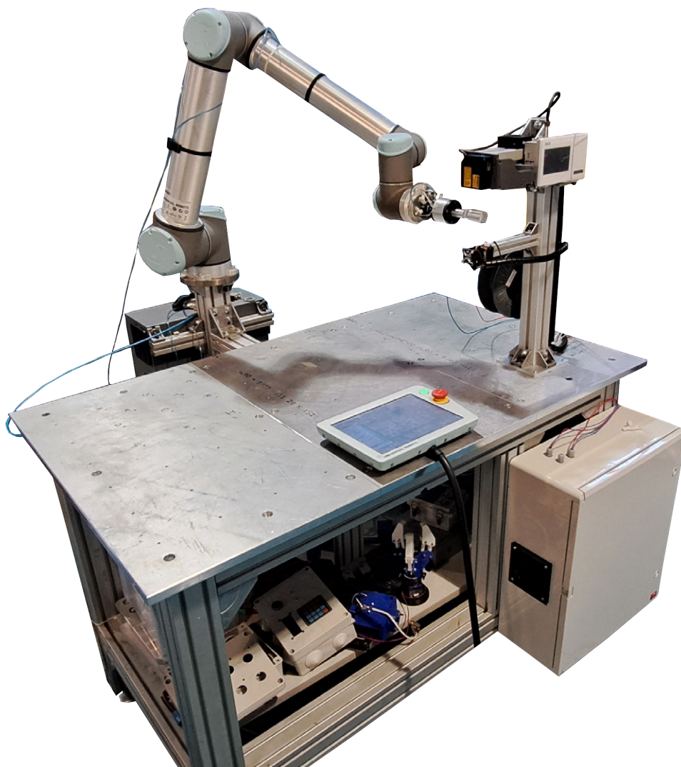
Figure 6.30: Robot-based NPAM-MEX-P manufacturing cell developed in this Thesis (isometric view).
