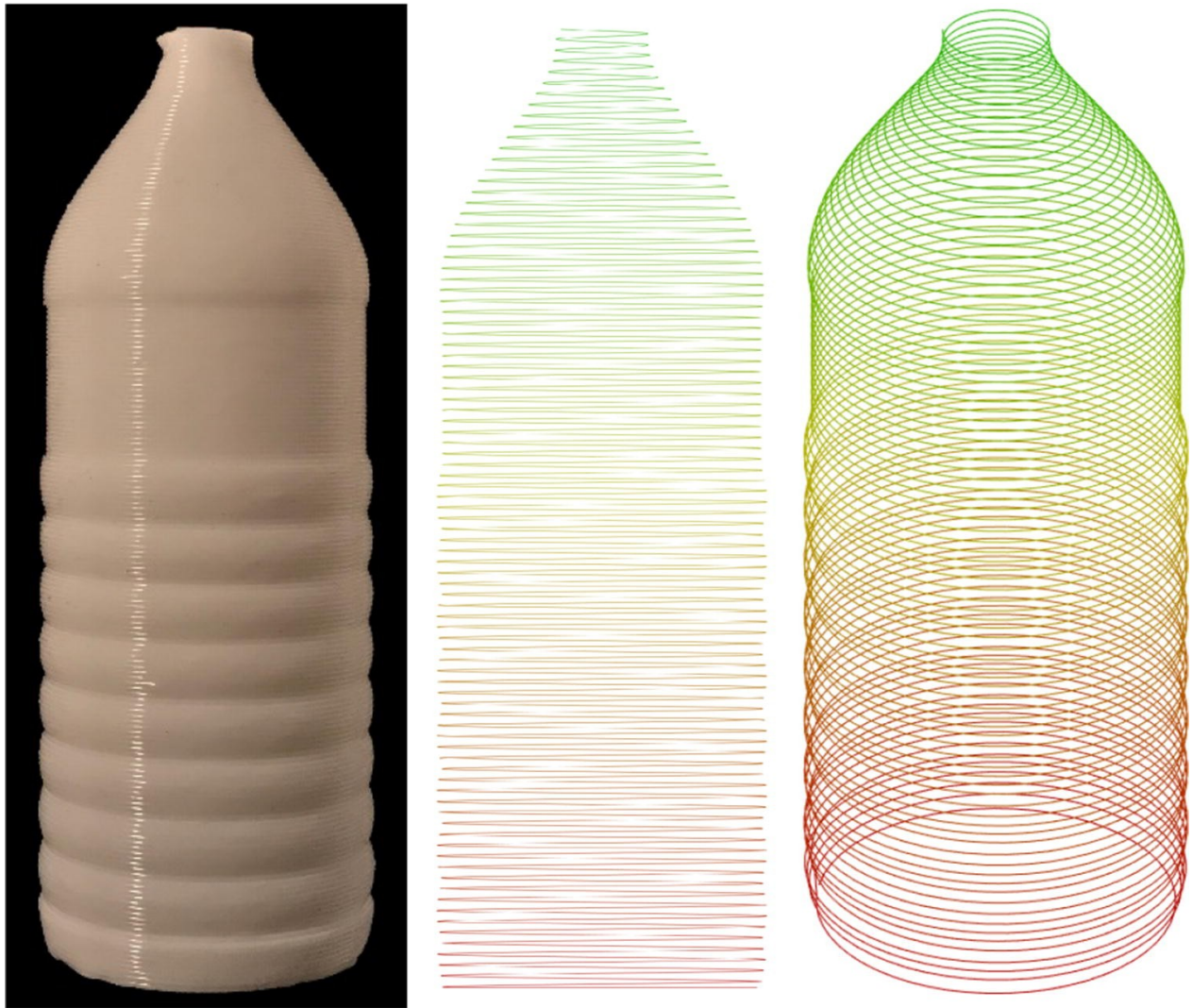
Figure 2.3: Helical shell slicing method [68]. Both the final result and the toolpath are shown.
