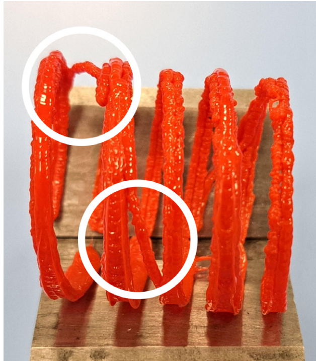
Figure 7.35: Travel moves with extrusion, highlighted in white.
