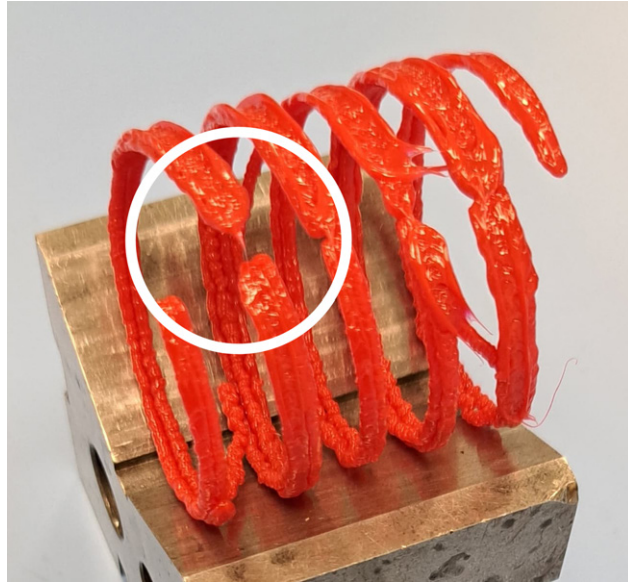
Figure 7.32: Build plate adhesion failure at the end of coil 1 (highlighted in white).
