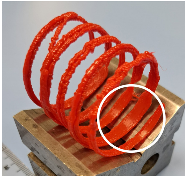
Figure 7.33: Build plate adhesion success at coils 3-5 (highlighted in white).
