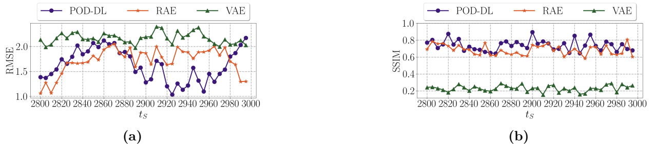
Figure 3.17: Error committed by the models, in each prediction for the streamwise velocity component, measured by the (a) RRMSE and (b) the SSIM.
