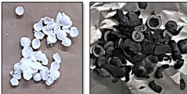
Figure 5.3: Prepared PLLA (left) and PLLA-AC (25% w/w) beads (right).
