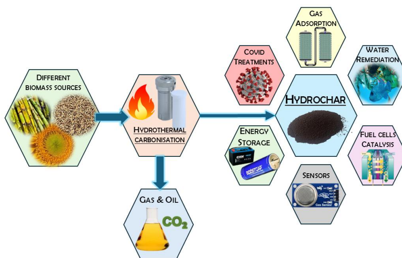
Figure 1.9: Schematic of HTC precursors, primary products and main applications of the produced hydrochar [172].
