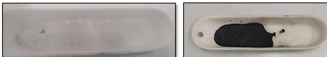
Figure 4.2: Residue after activation without (left) and with (right) pre-carbonisation step.
