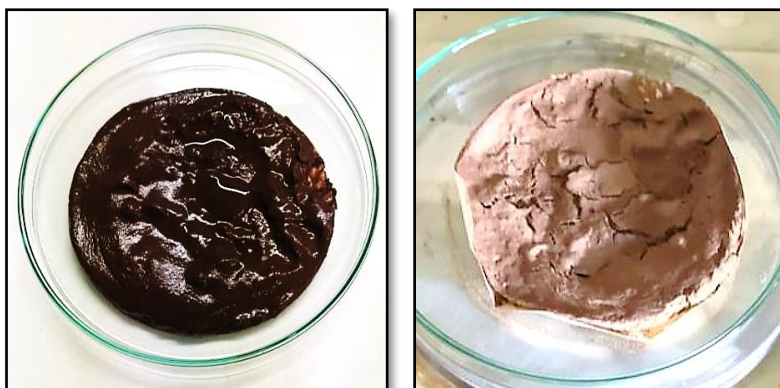
Figure 4.1: Obtained cellulose hydrochar (C200) before and after drying.
