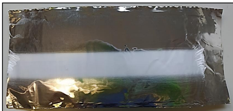
Figure 5.5: Electrospun PLLA-W fibre mat after 30 minutes.
