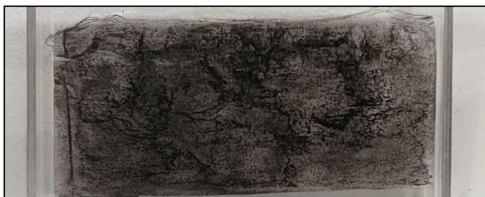
Figure 5.7: Final PLLA-W-AC fibrous structure.
