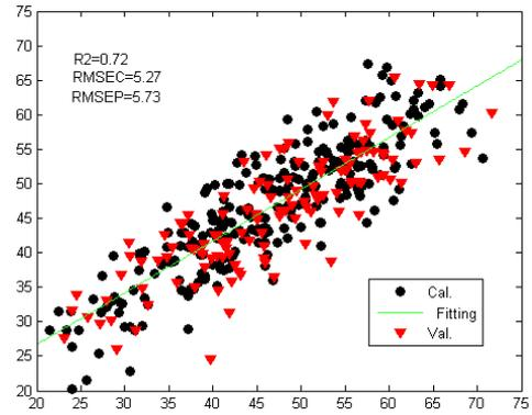
Fig. 4. MLR from mechanical and optical axis. Observed (x axis) against predicted MTF (y axis) and coefficient of determination ( $R^2$ ), Root Mean Standard Error of Calibration (RMSEC) and Root Mean Standard Error of prediction (RMSEP). Calibration (Cal.) and validation (Val.) populations are represented.
