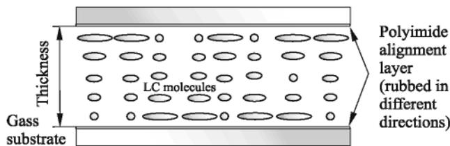
Fig. 8. Simple drawing of a security device LC cell. Glass substrates are coated with the polyimide alignment layer that induces different orientation in both planes to the LC molecules doped with a dichroic dye.
