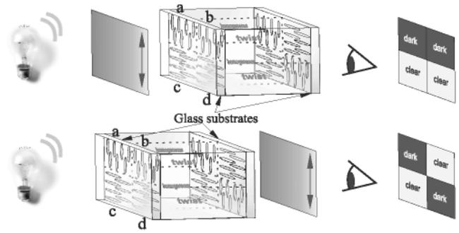
Fig. 2. Schematics of security device operating principle. Dichroic dye absorbs the light depending on orientation of LC molecules and polarization of light. Situation of polarizer determines which of two latent images is visible. Only an image generated on a substrate closest to a polarizer is seen.
