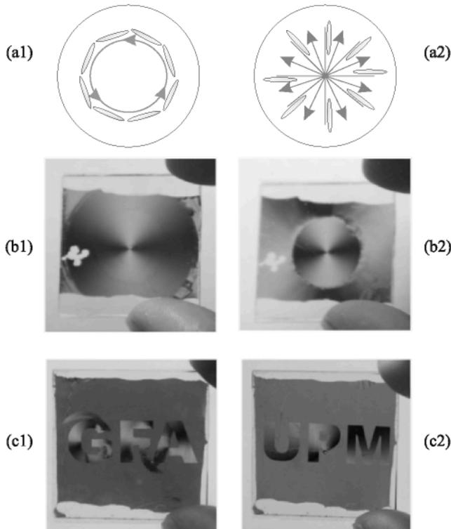
Fig. 6. Schematics of circular (a1) and radial (a2) rubbing direction, LC molecules are oriented according to this alignment. We can achieve continuous greyscales as in picture (b1) which corresponds to circular rubbing, and (b2) which is a combination of radial and circular rubbing. Pictures (c1) and (c2) show a combination of linear standard rubbing and circular rubbing.
