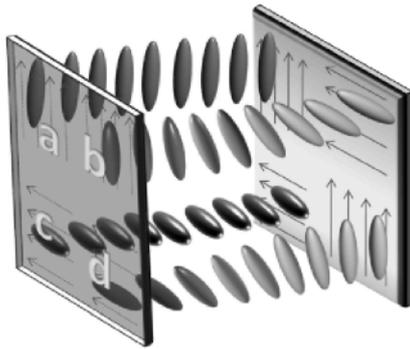
Fig. 1. A sketch of a simple LC security device. Alignment layers have been conditioned in order to induce different orientations on LC molecules generating the desired motifs. Twisted nematic structure allows creating different alignment patterns on each surface of one single device and makes it possible to create multiple latent images in the same device.
