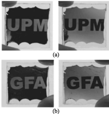
Fig. 3. Pictures of a device when a polarizer is placed in front of the LC cell (a) and when a polarizer is placed behind LC cell (b). Complementary images are obtained when a polarizer is rotated  $90^\circ$ .
