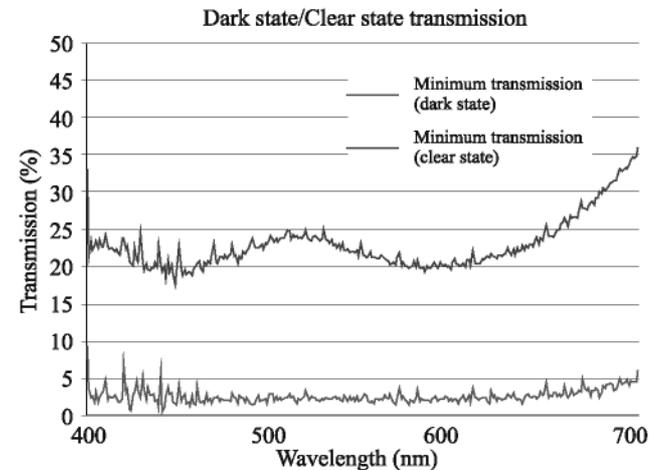
Fig. 7. Transmission obtained for one standard manufactured device in the case of dark state and clear state.
