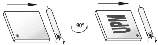
Fig. 4. Schematics of a rubbing procedure that allows “drawing” the latent motifs in a polyimide alignment layer. Firstly, a surface is rubbed in one direction and then, after a photolithographic process, a substrate is rotated  $90^\circ$  to change alignment of uncovered zones by rubbing again while maintaining remaining areas covered by a photoresist.
