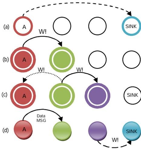
Figure 3 WSN with WuR: remote nodes communication
