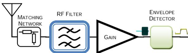
Figure 2 Generic Envelope Detector Receiver
