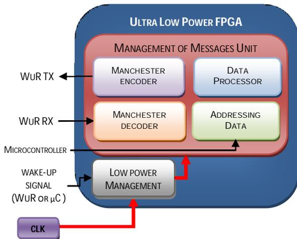
Figure 5 Wake-up scheme for *Flash\*Freeze* FPGA
