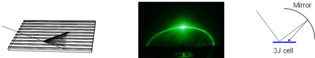
Figure 4 The irregularities and roughness of the gridlines of a commercial concentration triple-junction cell has approximately cylindrical symmetry, which allows efficient external confinement with an asymmetric cavity.
