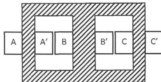
Figure 1: Conventional three-phase transformer with planar windings
