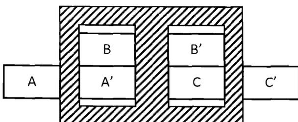
Figure 2: Proposed three-phase transformer with planar windings
