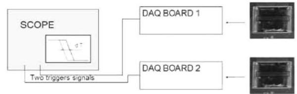
Fig. 2. Scheme of the set-up used to evaluate the time coincidence distribution.
