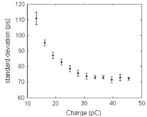
Fig. 3. Standard deviation of the time delay distribution as a function of the charge injected.
