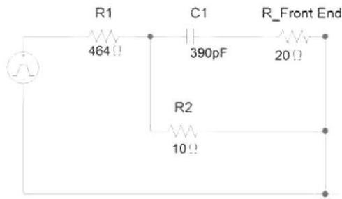
Fig. 1. Schematic of the charge injection circuit where the  $20\ \Omega$  impedance symbolizes the Front-End contribution.
