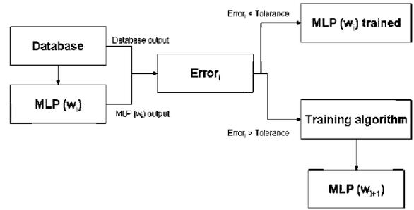
Fig. 2. Adjusting of weights of a MLP. Scheme of the learning process for a MLP. The database is the set of examples used to train the MLP.
