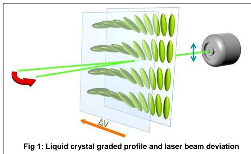
**Fig 1: Liquid crystal graded profile and laser beam deviation**
