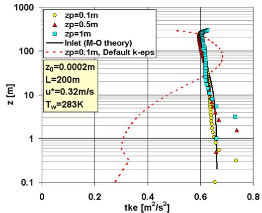
Figure 4: Near-wall grid sensitivity on the profile. Comparison with default model configuration.
