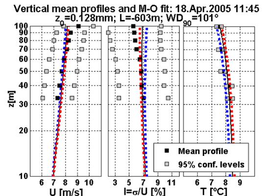
Figure 8: Unstable case mean velocity and turbulence intensity profiles with M-O fit.
