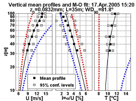
Figure 7: Stable case mean velocity and turbulence intensity profiles with M-O fit.
