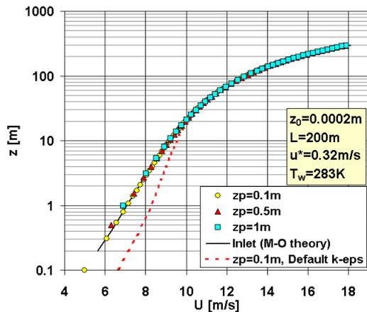
Figure 2: Near-wall grid sensitivity on velocity profile. Comparison with default model configuration.
