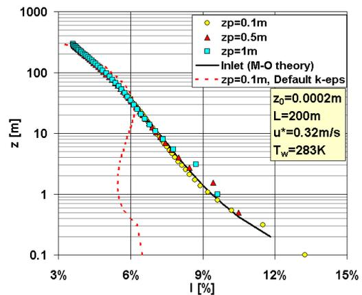
Figure 5: Near-wall grid sensitivity on turbulent intensity. Comparison with default model configuration.
