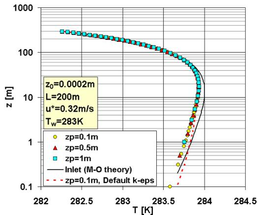
Figure 3: Near-wall grid sensitivity on temperature profile. Comparison with default model configuration.
