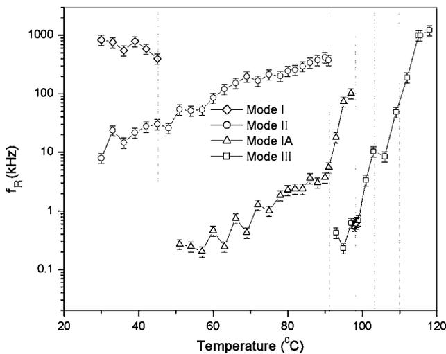
FIG. 7. The variation of relaxation frequency ( $f_R$ ) with temperature for 4  $\mu\text{m}$  cell thickness during heating.
