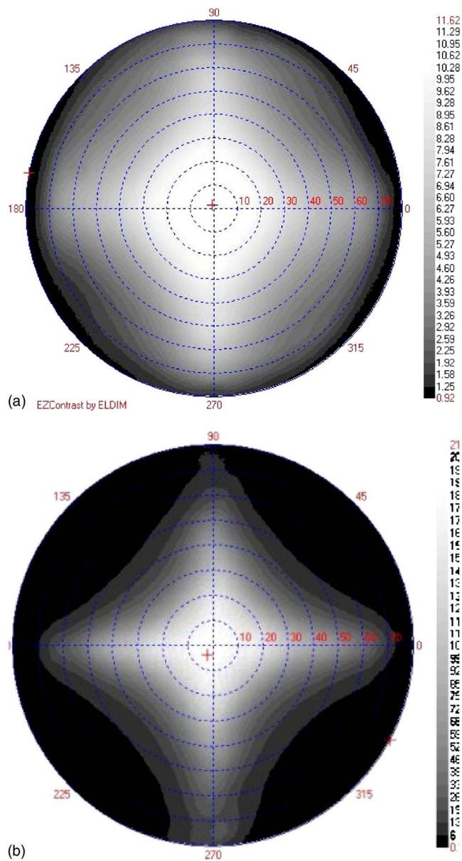
FIG. 2. (Color online) (a) Isocontrast plot measured with an ELDIM EZ-contrast system on the cell filled with CS-4001. (b) Isocontrast plot measured with an ELDIM EZ-contrast system on the cell filled with W-182.
