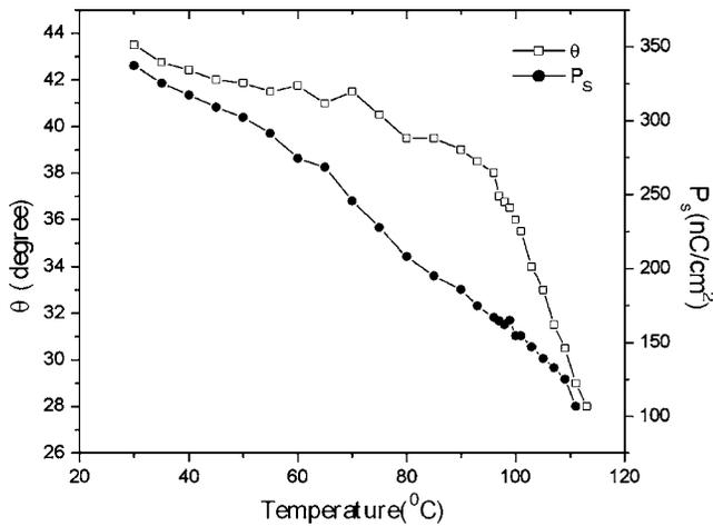
FIG. 4. The variation of tilt angle ( $\theta$ ) and the spontaneous polarization ( $P_s$ ) of W-182 OAFLC molecules with temperature for  $4 \mu\text{m}$  cell thickness.
