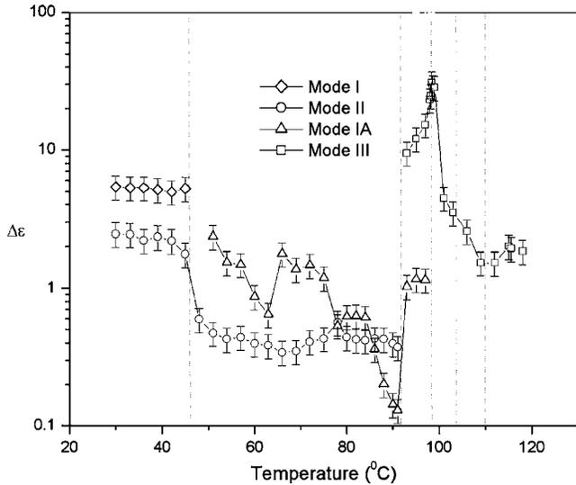
FIG. 6. The variation of dielectric strength ( $\Delta\epsilon$ ) with temperature for 4  $\mu\text{m}$  cell thickness during heating.
