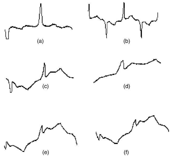
FIG. 5. The polarization response current peaks obtained at different temperatures during heating of the studied OAFLC for  $4 \mu\text{m}$  cell thickness: (a)  $30^\circ\text{C}$ , (b)  $55^\circ\text{C}$ , (c)  $80^\circ\text{C}$ , (d)  $100^\circ\text{C}$ , (e)  $105^\circ\text{C}$ , and (f)  $109^\circ\text{C}$ .
