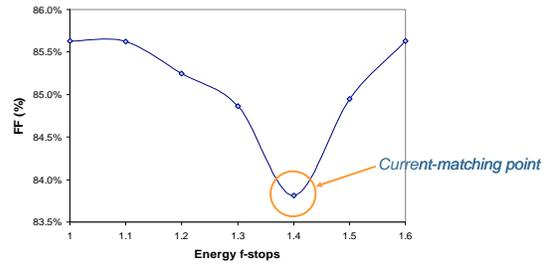
Figure 5. FF of a 3J cell from Spectrolab at constant  $I_{sc}$ , as a function of the flash pulse energy. The higher the energy, the more blue-rich the spectrum is.
