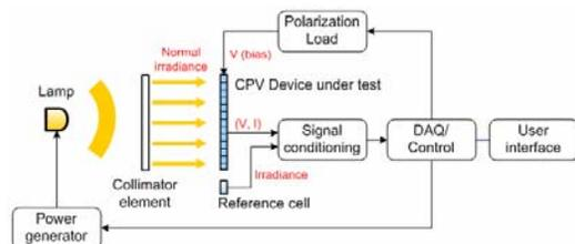
Figure 3. Elements of the multi-flash CPV solar simulator.
