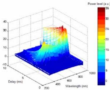
Figure 4. Spectrometer measurement of the Xenon light source intensity as a function of time from peak.
