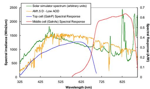
Figure 6. Solar simulator spectrum for a specific triggering voltage at peak power compared to AM1.5D standard spectrum. Also, spectral responses from top and middle junctions in a typical triple-junction cell are shown.
