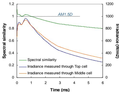
Figure 7. Spectral similarity through current ratios of top and middle component cells (GaInP, GaInAs) under solar simulator and reference AM1.5D conditions. It is given as a function of time, during the flash pulse decay. Available irradiance for top and middle cells is measured using Eq. 1
