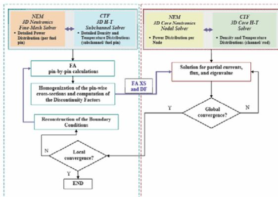
Fig. 2. Multi-scale and multi-physics coupling in the PSU code system
