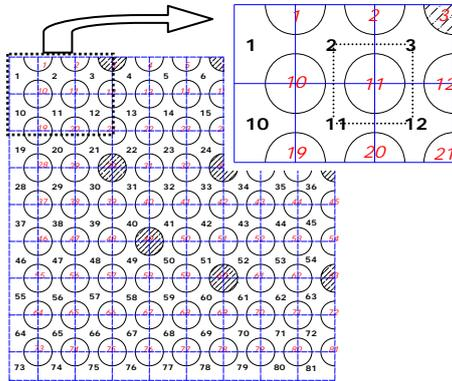
Fig 5. Coupling discretization scheme at pin cell level
