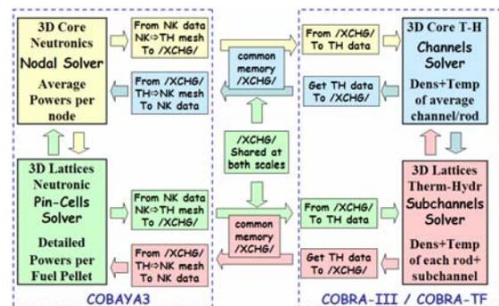
Fig. 1. Multi-scale and multi-physics coupling in the UPM code system.
