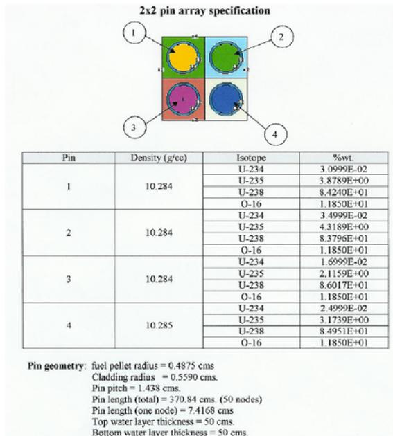
Fig. 3. 2x2 pin array test problem specifications
