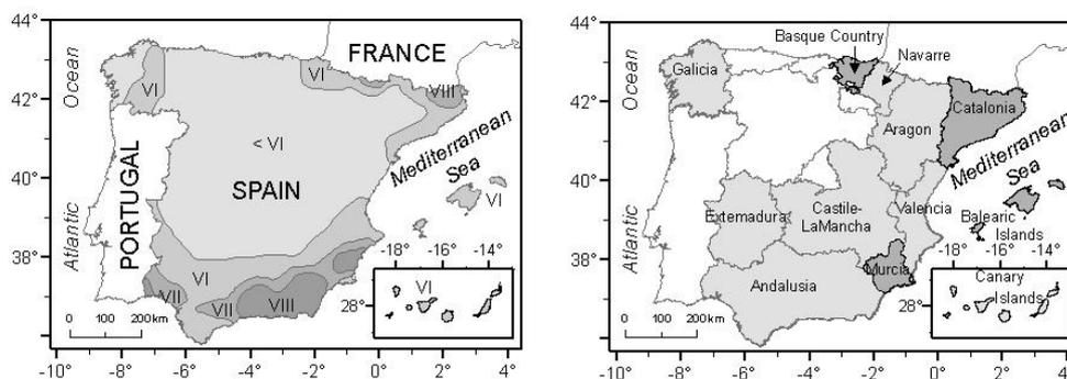
Figure 1 Left: DBPPCRS seismic hazard map of Spain (DBPPCRS, 2004); right: regions (in grey) that must develop specific regional seismic risk studies (regions with already accredited plan are shown in dark grey).
