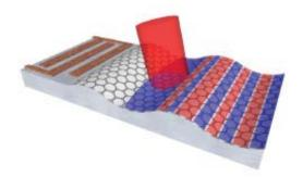
**Figure 1:** A sketch of our proposed device to couple laser light into propagating graphene plasmons.
