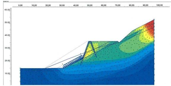
Figure 8. Elimination of the mass of ground in front of the row of micropiles. Embedding in the substrate: 3.5 m.
