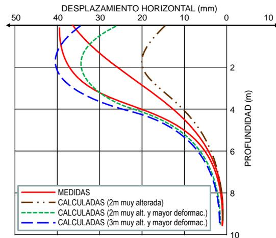
Figure 12. Comparison of real and calculated measurements (horizontal movements)
