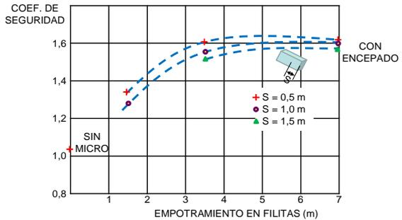
Figure 9. Influence of embedding in the substrate on the safety coefficient.
