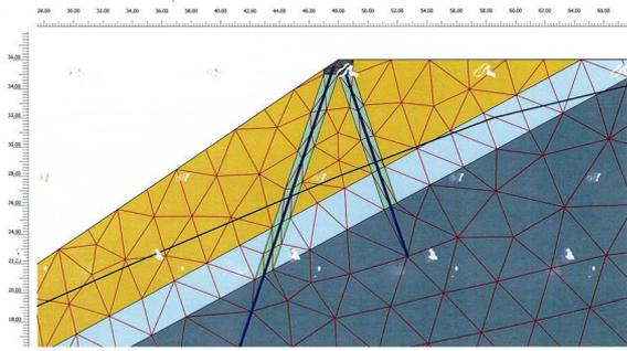
Figure 5. Mesh with beam element. High water table (F=1.15).
