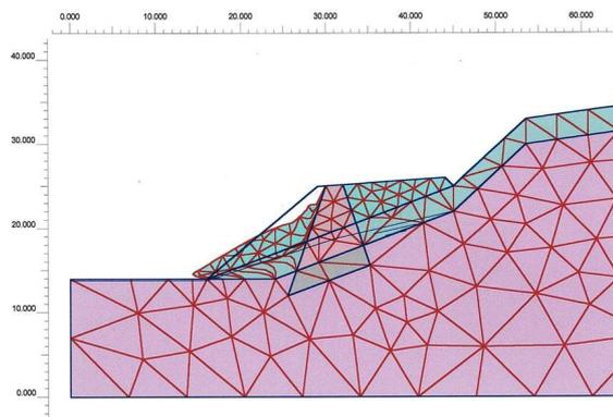
**Figure 4.** Breakage in the case of the improved zone and lowering of the water table
