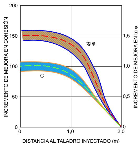
**Figure 2.** Hypothesis on improvement of the terrain around an injected micro
