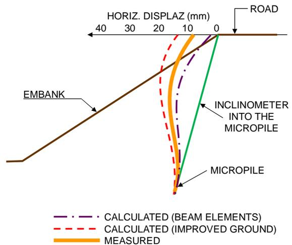
Figure 7. Comparison of calculated and measured movements in Ceuta.
