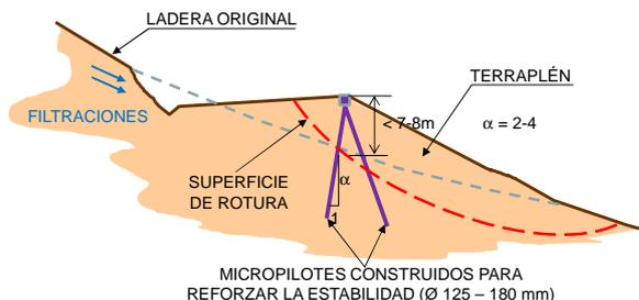
**Figure 1.** Case of an increase in stability of embankments on a hillside (vertical piles plus various inclinations)
