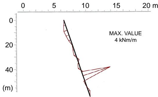
Figure 6. Law of bending moments in the pile furthest from the slope of the embankment.
