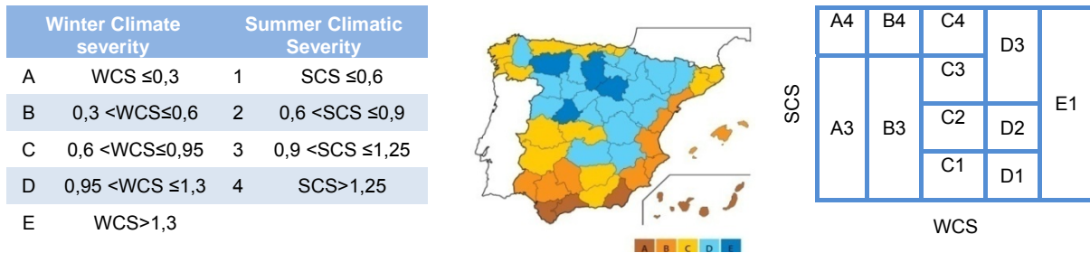
Figure 4. Spanish Building Code Climatic Classification
