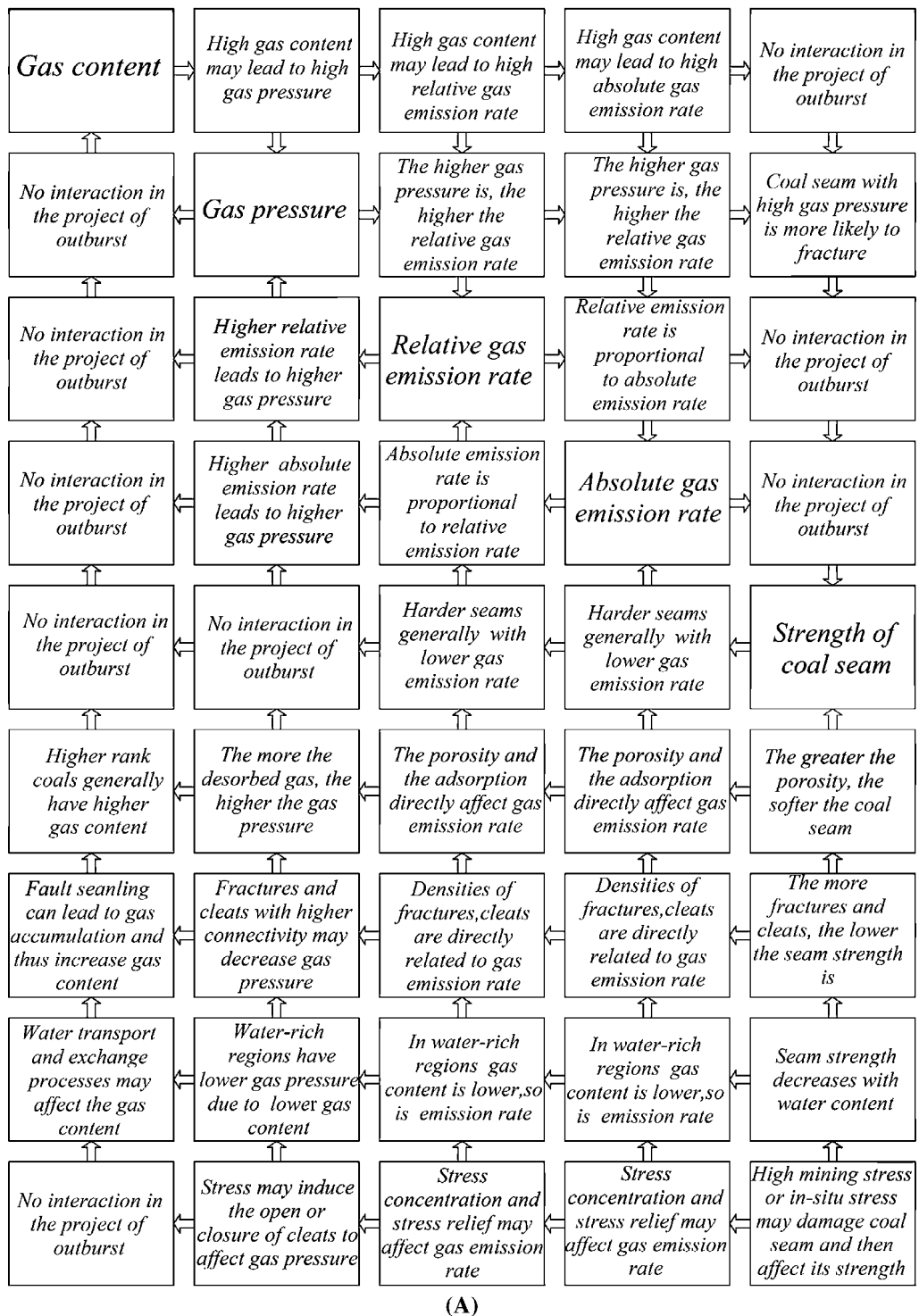
Figure 3. The constructed interaction matrix of the coal and gas outburst system. Note: A is the left part of the matrix and B is the right part of the matrix.
