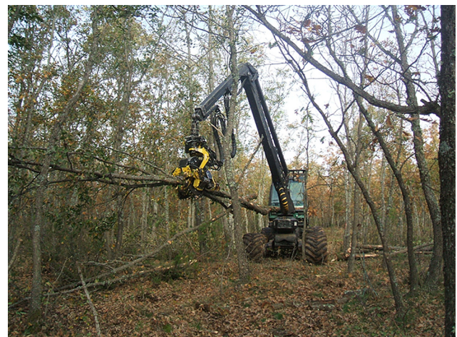
Fig. 1 – Multi-tree forest harvesting felling a Quercus coppice stand (WTH3).
