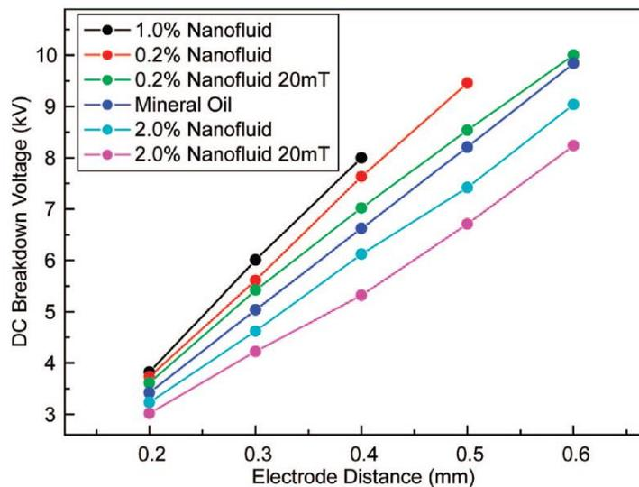
Figure 7. DC breakdown voltage compared with electrode distance for mineral oil and different concentrations of Fe<sub>3</sub>O<sub>4</sub> oil-based nanofluids, some of them are subjected to a 20 mT external magnetic field [1] adapted from [27]
