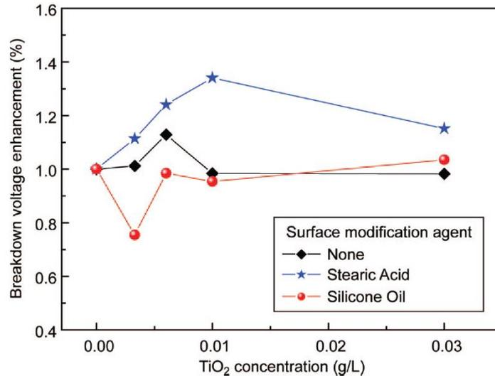
Figure 6. AC breakdown voltage dependency of surfactants for different mineral oil-based TiO<sub>2</sub> nanofluids compared with different TiO<sub>2</sub> concentrations [1] adapted from [26]
