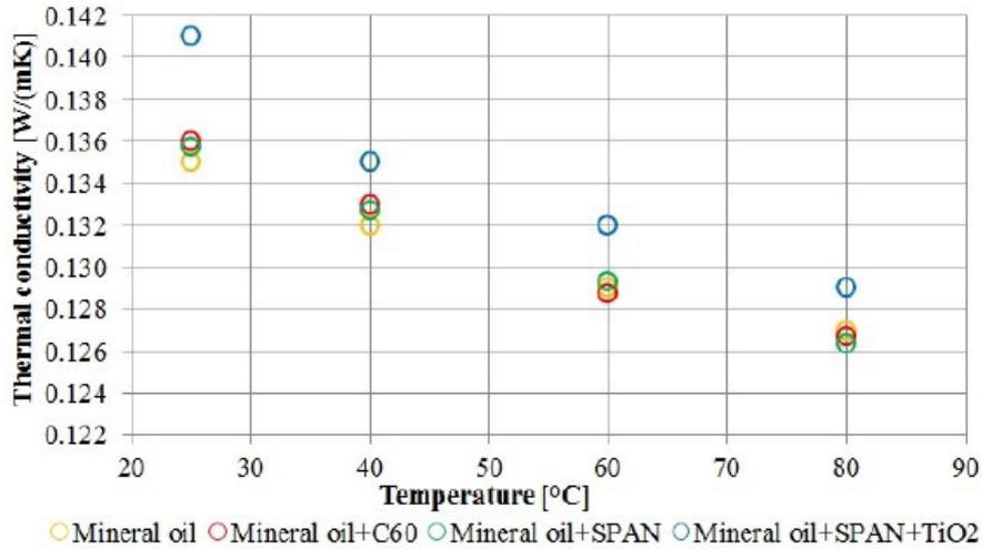
Figure 3. Thermal conductivity coefficient of mineral oil and nanofluids formed on its basis, as a function of temperature. Take from [6]
