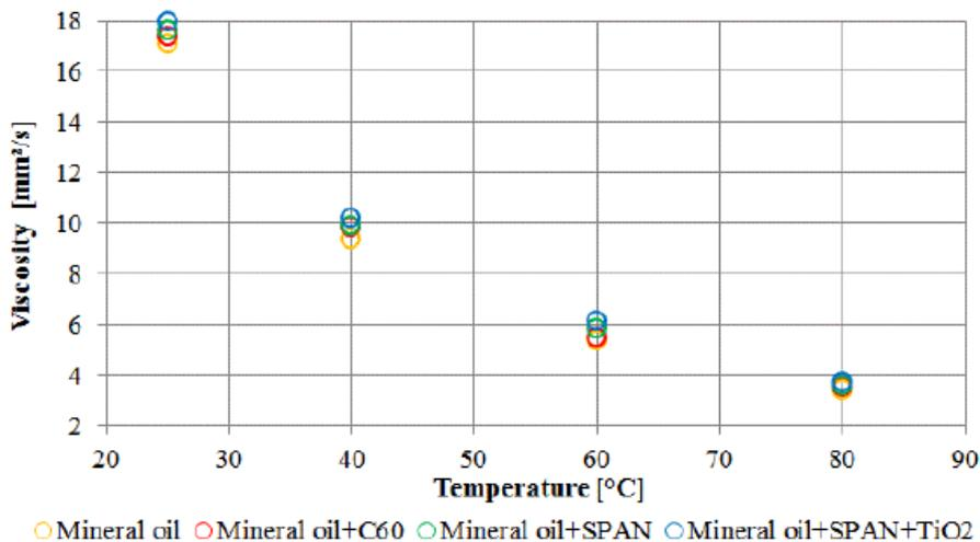
Figure 4. Viscosity of mineral oil and nanofluids formed on its basis, as a function of temperature. Taken from [6]
