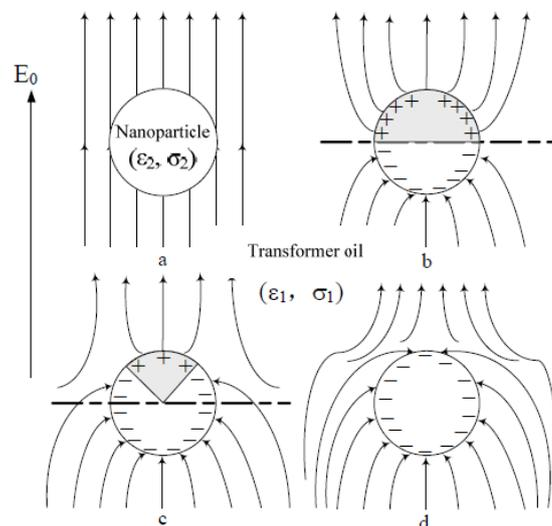
Figure 2. Electric field lines after a uniform z-directed electric field is activated at  $t = 0$  around a Nanoparticle with radius  $R$ , permittivity  $\epsilon_2$ , and conductivity  $\sigma_2$ . This nanoparticle is surrounded by transformer oil with permittivity  $\epsilon_1$  and conductivity  $\sigma_1$ . Taken from [2]
