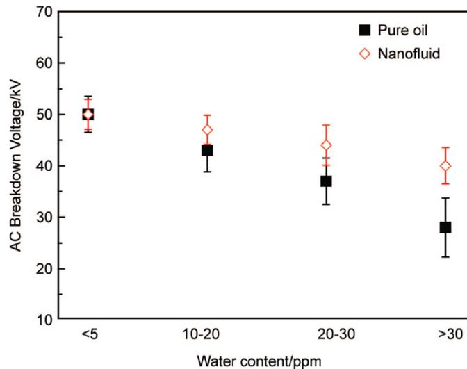
Figure 5. AC breakdown for mineral oils and  $Fe_3O_4$  mineral oil-based nanofluids as function of water content. Taken from [1] that adapted it adapted from [13]
