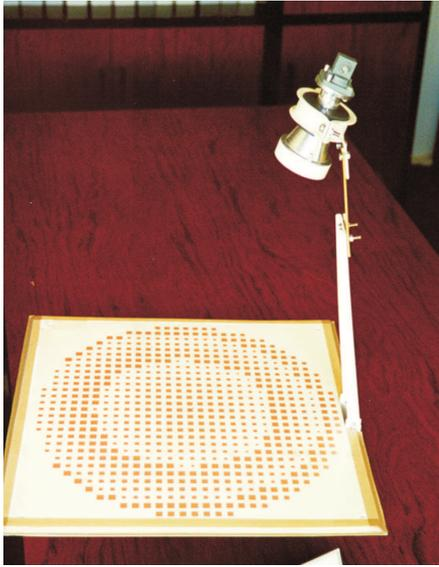
Figure 1: Photograph of a reflectarray antenna fed by a conical corrugated horn.
