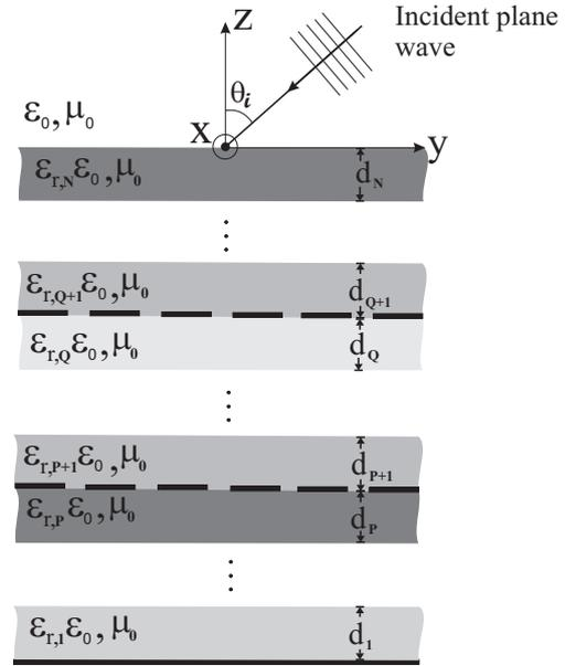
Figure 2: Scattering of a plane wave by a multilayered substrate containing several infinite periodic arrays of microstrip patches.
