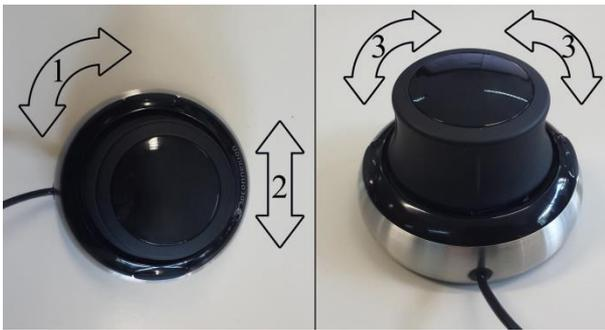
**Figure 1.** 3D mice used as endoscope controllers. On the left, 3D mouse for the left hand controlling rotation motion (1) and insertion motion (2). On the right, 3D mouse for the right hand responsible for flexion motion (3).
