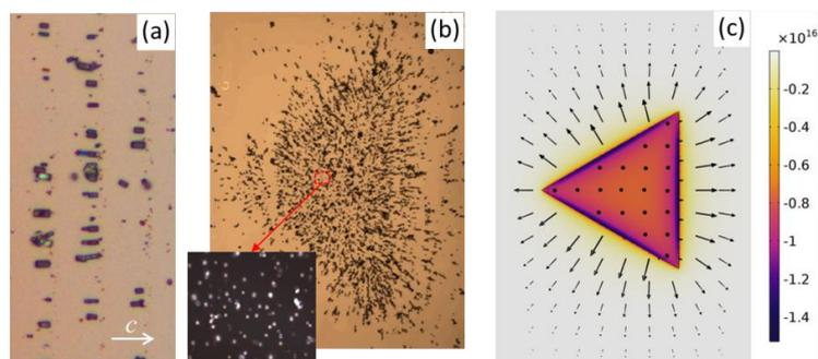
Figure 1: (a) ZL fringe pattern obtained by illuminating a  $x$ -cut sample with a sinusoidal pattern with  $\lambda=18$   $\mu\text{m}$  periodicity, (b) ZL triangle pattern obtained in a  $z$ -cut sample illuminating with a triangle light image (800  $\mu\text{m}$  side). (c) Simulation of the evanescent PV field (arrows) and DEP potential (colour degrade) for the experiment of the triangle. In both cases, ZLs are aligned along the evanescent electric field lines.
