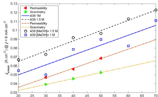
Figure 1. Predicted crossover at 8 mA·cm<sup>-2</sup> and several temperatures (○ 1.5 M methanol, □ 1 M methanol polarization curves). ◀ Calculated crossover from permeability measurements (1 M methanol) [5]. ▶ Calculated crossover from CO<sub>2</sub> production gravimetric measurements (1 M methanol) [5].
