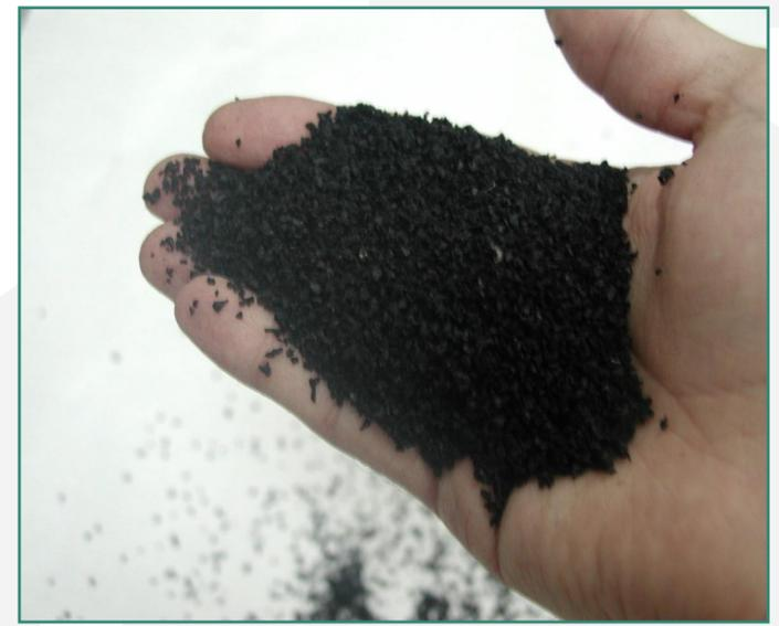
**Fig. 1** Commercial ground tyre rubber used as starting material.
