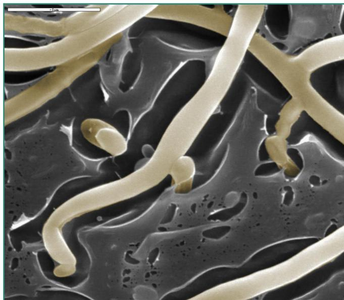
**Fig.2** Low temperature scanning electron microscopy (LT-SEM) image of the fungus growing inside the commercial ground tyre rubber.
