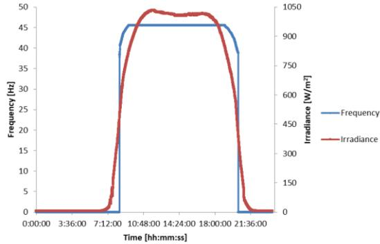
**Figure 7:** Pump Frequency related with the irradiance received by the PV generator (2<sup>nd</sup> June 2017).
